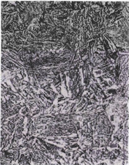
FIGURE 4-30 Alloy 4340 normalized at 871°C for 1 h and air-cooled; structure consists of upper bainite. (Etch: 2% nital; 400×.) (Courtesy of Republic Steel Co.)
