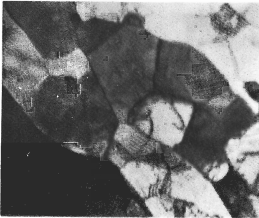
FIGURE 2-28 Recovered structure of Fe-0.18% C martensite after tempering 10 min at 600°C; electron transmission micrograph. (Thin-foil specimen: \times 30,000 .) [After G. R. Speich and W. C. Leslie, Metall. Trans. 3(1972):1043.]
