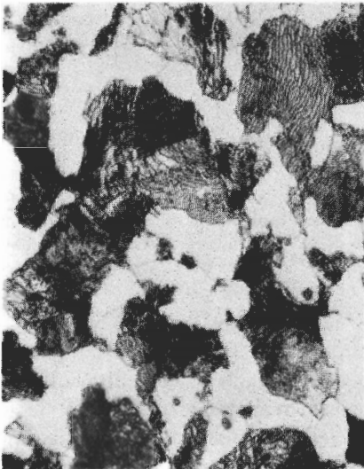
FIGURE 4-25 Alloy 4140 steel fully annealed 24 h at 691°C; structure consists of pearlite with ferrite. (Etch: 2% nital; 800 ×.) (Courtesy of Republic Steel Co.)
